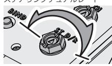
To be used to adjust steering servo throw.
