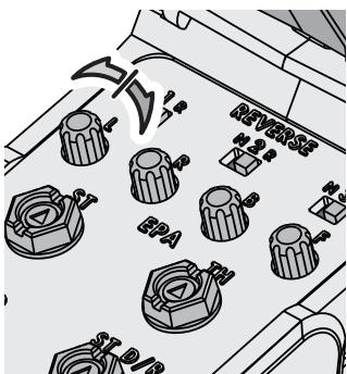
**End point adjustments allow you to set the limits of steering and throttle.**
